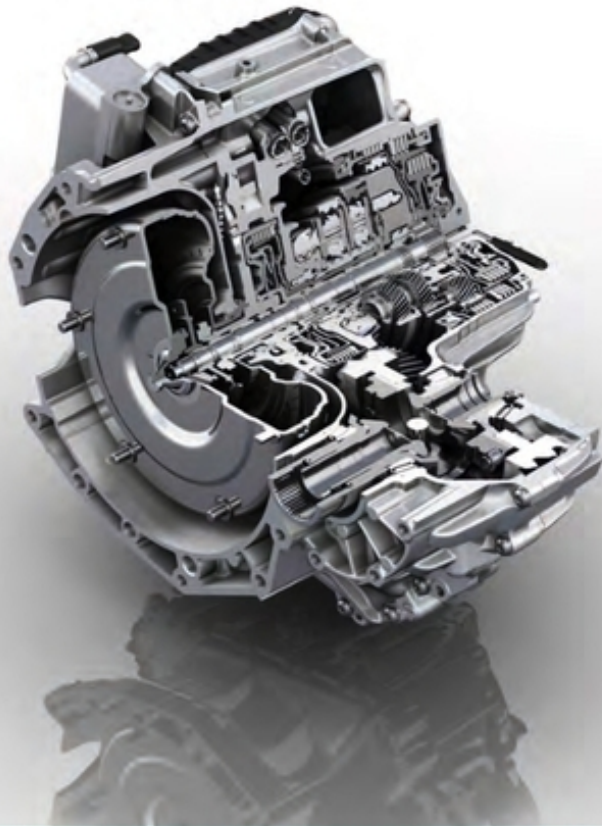
Figure 2: An example of an advanced 9-speed automatic transmission design
